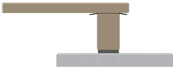
Example of use of a moisture barrier. Spacer block between concrete slab and joist. Suitable sill tape between joist and decking.
