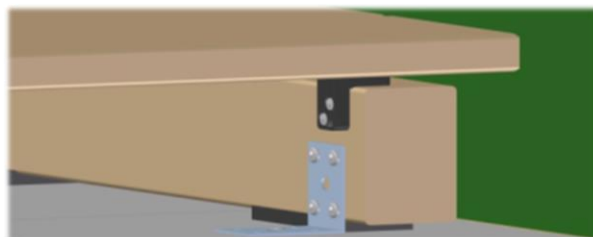
Figure 8: Screw the end clip to the substructure.
