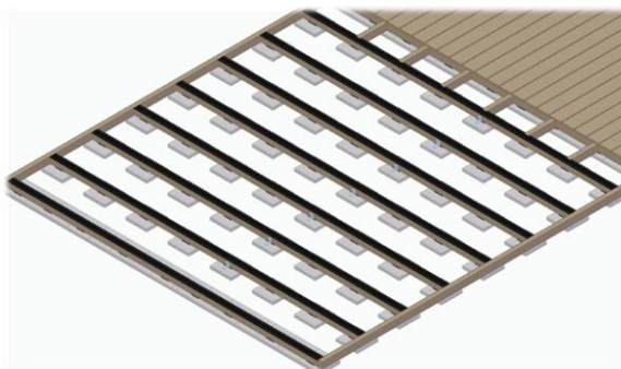
Joist tape used between decking and joists.
