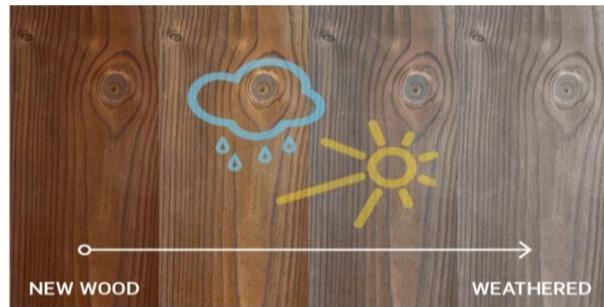
The Kebony technology gives the wood a deep rich brown colour (some natural colour variations will occur and there are possible darker areas as a result of the process). After exposure to sun and rain the wood will develop a natural silver-gray patina where surface cracks and checks may appear, this is a natural development and will not influence the performance and durability of the wood.
