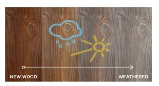
The Kebony technology gives the wood a deep rich brown colour (some natural colour variations will occur and there are possible darker areas as a result of the process). After exposure to sun and rain the wood will develop a natural silver-gray patina where surface cracks and checks may appear, this is a natural development and will not influence the performance and durability of the wood.
