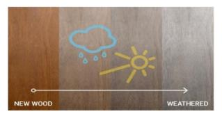
The Kebony technology gives the wood a deep rich brown colour (some natural colour variations will occur and there are possible darker areas as a result of the process). After exposure to sun and rain the wood will develop a natural silver-gray patina where surface cracks and checks may appear, this is a natural development and will not influence the performance and durability of the wood.
