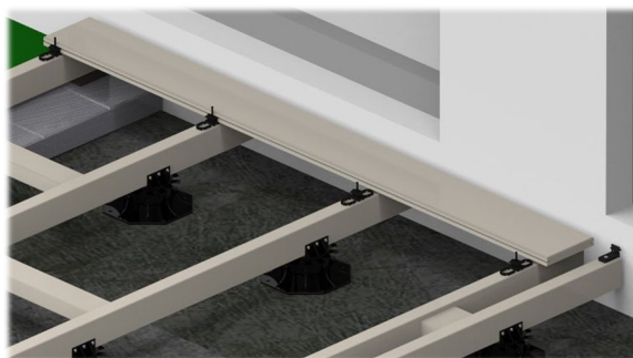
Figure 16: First board. Do not screw the decking clips in before the next board is correctly placed.
